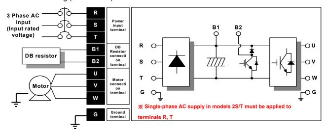
Power terminal wiring (11.0 ~ 22.0kW)
