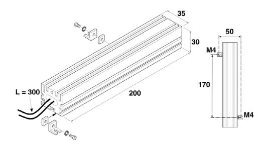
Overall Dimensions, Resistor 350W - IP55
