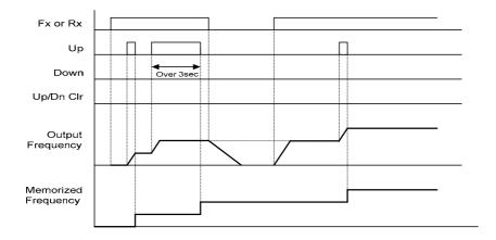
▶ When F65 is 2: It is increased as much as step frequency set as F66 at the rising edge of multi-function input set as UP and if it is activated for 3 seconds, it operates as it was set as "0". It is decreased as much as the step frequency set as F66 at the rising edge of multi-function input set as DOWN. If it is activated for 3 seconds, it operates as it was set as "0" and the accel/decel time is the same as when set as "0".
