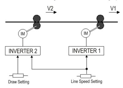
$$T = E \times S \times D = E \times S \times \frac{V1 - V2}{V2}$$
