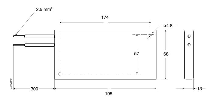
Overall Dimensions, Resistor 550W - IP55
