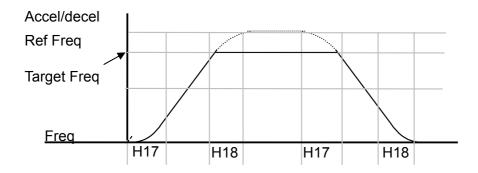
Frequency is below Max Frequency, the waveform will be shown with the top portion cut out.
