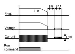
▶ In case of DC brake at high load inertia and frequency, change the DC brake controller gain according to H37 set value.
