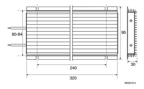
Overall Dimensions, Resistor 1100W – IP55
