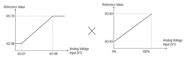
$$FBK \ display = \left( \left( \frac{I10 - I8}{I9 - I7} \right) \times \left( Input \ Voltage - I7 \right) + I8 \right) \times \frac{(I90 - I89)}{MaxFreq} + I89 \quad when \ feedback \ is \ from \ V1$$
